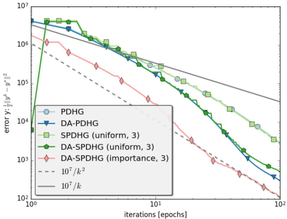
Figure: Distance to dual part of the saddle point.
