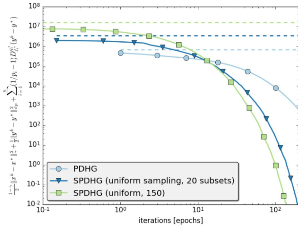
Figure: distance to a saddle point
